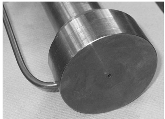
Fig. 2 The aperture collar shielding the DPV-2000 sensor window
